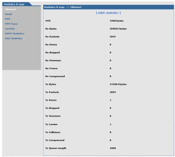
This is an example of the Ethernet Statistics & Logs screen. It shows Ethernet statistics.
